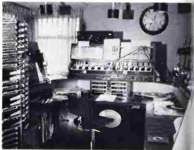
This is the Master Control Room. The five pots, 25-button extender panel on the Sparta console (right side) eliminates need for patch panel. The six ITC cart machines operate in sequence.
