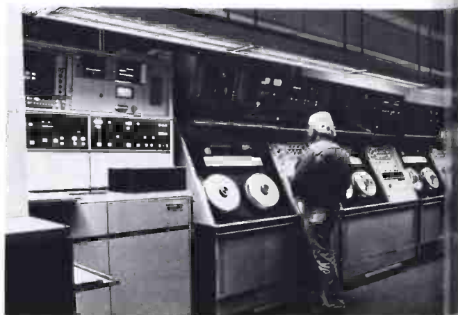
Production area, with three of station's Ampex AVR-1's in view.
