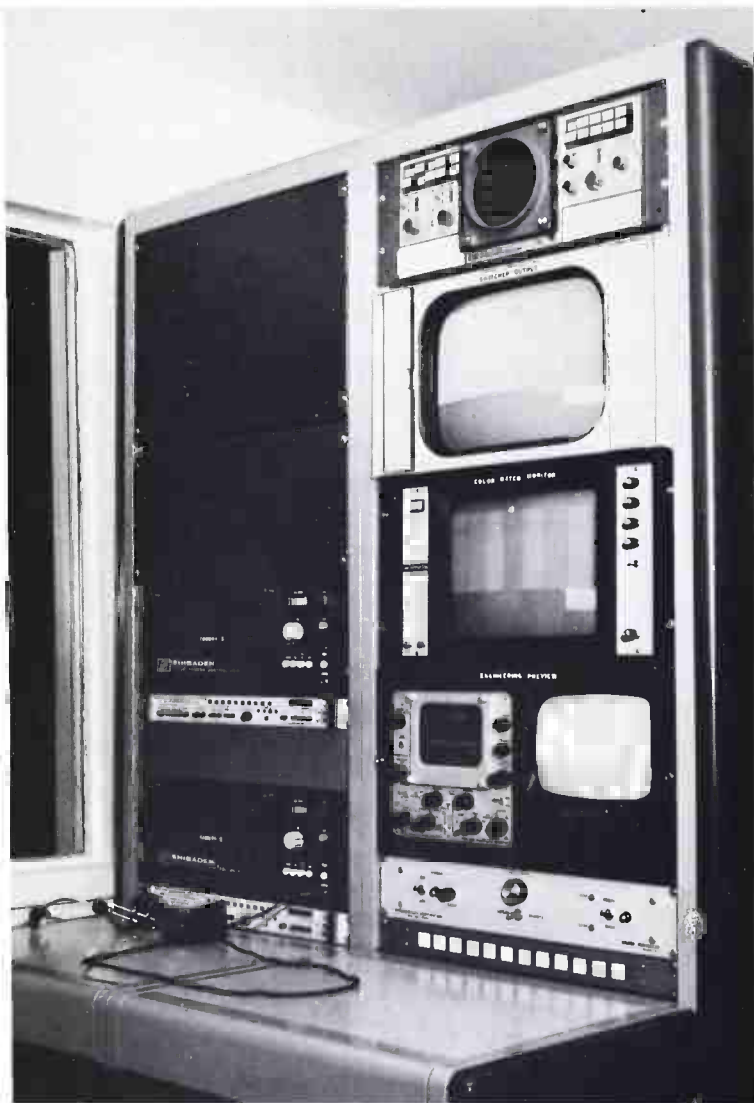
Color control racks include digital color encoder and imager enhancers to upgrade Shibaden FPC-1000A cameras.
